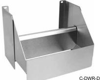
The C-DWR-D model is 10" deep frontto-back and designed to align with adjacent equipment that has a double speed rail. The C-DWR-D has a speed rail step in the back with the dry waste chute at the front.
