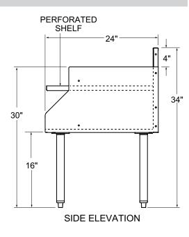
Recessed drainboards have the same corrugated work surface as normal drainboards except the work surface has been lowered to allow stacking of glassware. A perforated shelf is placed on top of the first level of glassware and a second layer of glassware is stacked on top of it. Recessed drainboards work best when only one style of glassware is being stored.
