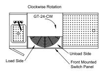
**2. ROTATION:** Conveyor rotation can be clockwise or counterclockwise. The rotation selection is based on work flow. In an underbar environment, the wet waste sink should be on the load side of the glass-washer to prevent crossover (see underbar plan view). In a pass-thru style cocktail station, the load side should be toward the servers (see pass-thru station plan view).
