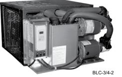
Which line chiller size should you choose? Remote beverage line chillers are sized to handle different length runs. If two separate conduits are involved, then the lengths of the two runs must be added together to determine the total run requirement. The run length is calculated as the distance between the line chiller and the beverage tower in a single pass glycol conduit, including any rise or fall.
