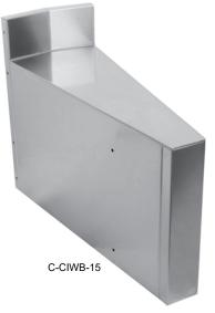
\*NOTE: Choice Corner Inside Wedge Fillerboards are manufactured to order and are not returnable Corner inside wedge fillerboards are all 24" deep and available for small degree inside turns. Corner fillerboards are designed to mount between two pieces of Choice underbar. However, corner fillerboards can be used to mount between any two stable vertical surfaces. Corners should not be mounted to objects that are mobile or on casters.
