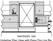
Underbar Plan View with Pass-Thru Ice Bin and Back-to-Back Mounted Underbar
