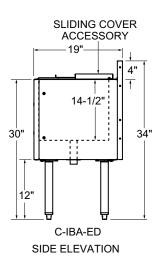
NOTE: Ice bins intended to store potable ice must be ordered with an ice bin cover to maintain the sanitation listing
