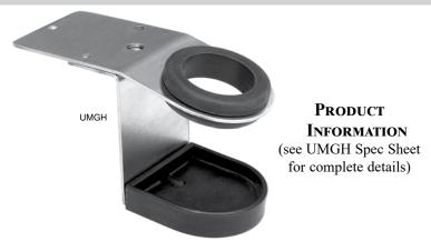
14 gauge stainless steel with rubber grommet and plastic drip pan. Grommet is specially sized to properly hold both Wunder-Bar® and Schroeder America<sup>TM</sup> style soda guns. Includes 10' of drain line tube.
